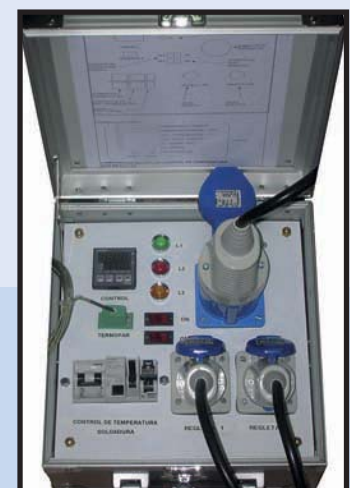
Fig. 3G: Control maquina de soldar PTFE Heat sealer control
